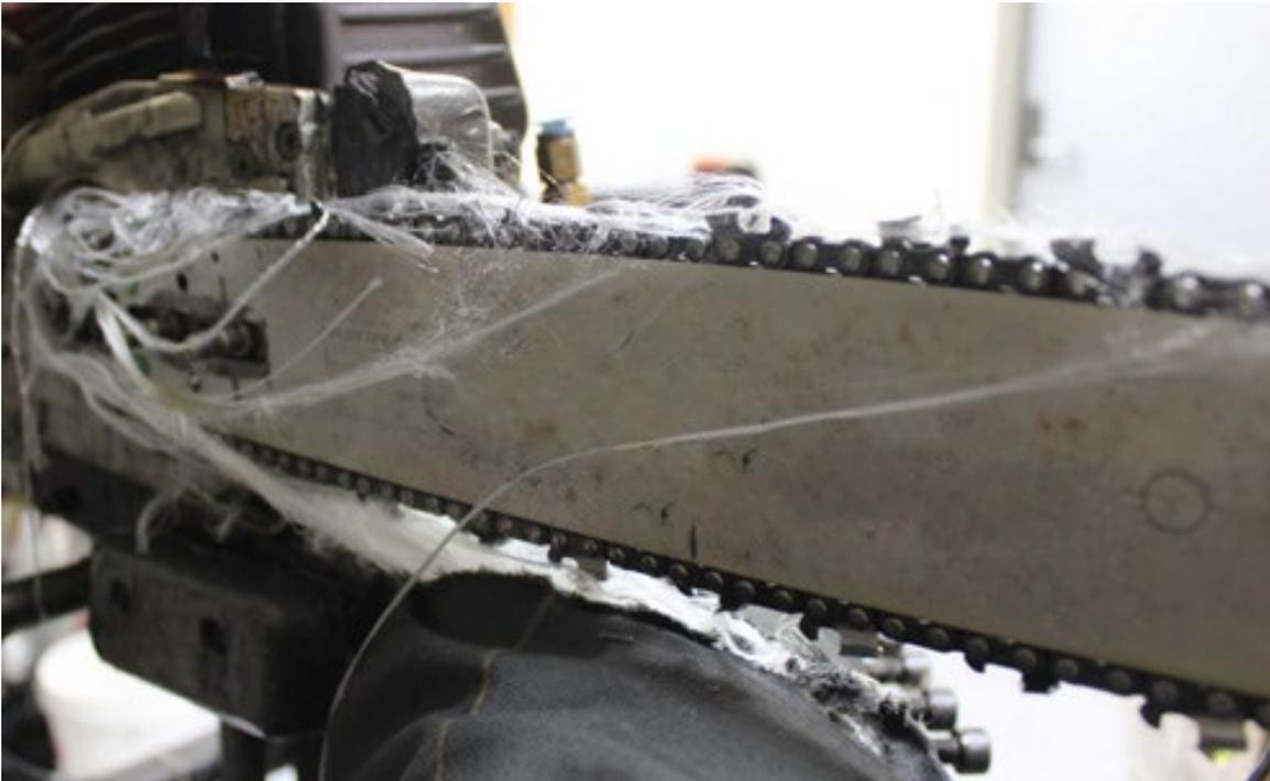
When a chainsaw chain hits this mat **the teeth act like hooks**, dragging these fibres out, which then get tangled around the sprocket, **choking it**.
